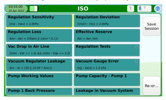
You can perform the test steps in any order, subject to any preconditions/test results that a given step may need. DTX will have a natural testflow to move through steps in the listed order, ie, when one step is completed it will move on to the next uncompleted step.
