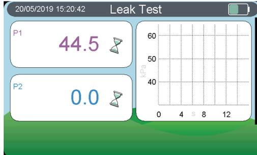
The screen will show an hourglass if the vacuum is not above 45kPa. When the vacuum is high enough a 'play' button will appear. Press the button and the test will start.
